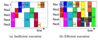
Figure 4. Illustration of the metric of resource use rate
