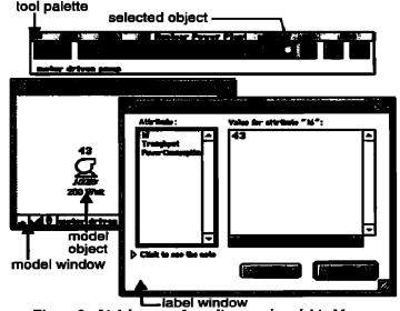
Figure 2 : Link between formalisms and model in Macao. Figure 2 illustrates the relation between a formalism description and related models. Classes declared in the formalism are described in the tool palette (top of Figure 2). Users can select one of them and create instances in the model (a model object) in a window that contains a model description (bottom left in Figure 2). It is then possible to edit labels related to this objects and declared in the corresponding class description.
