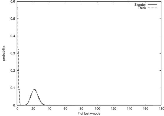
Fig. 6: Loss quantity versus probability for a given 512 p-nodes system with degree 4 : 8
