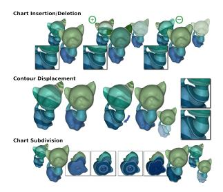
Fig. 5. Global impact of Reeb atlas editing operations. Reeb charts whose triangle list changes after the operation are transparent. Top: chart insertion and deletion (through insertion and deletion of extrema). Middle: contour displacement. Bottom: chart subdivision.
