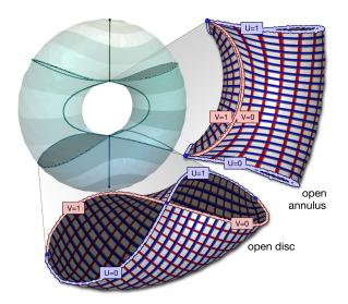
Fig. 3. Our parameterization strategy maps the boundaries of the Reeb chart (open annulus or open disc) to the unit square by defining UV Dirichlet boundary conditions within the Laplace system. Open annuli are cut into discs by a streamline guided by the scalar field gradient.
