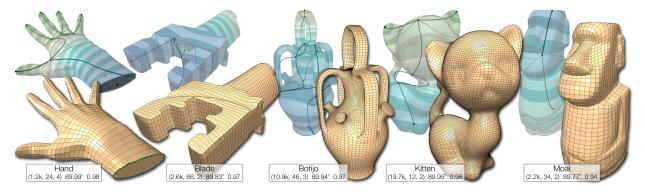
Fig. 14. Examples of user designed quad meshes generated with our framework accompanied by quality statistics (vertex count, extraordinary vertex count, max difference from the valence-4, the average mesh angle and scaled Jacobian).
