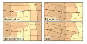
Fig. 12. T-junctions are resolved by the stitching process: inserting new quads where multiple T-junctions share a common edge (a), or performing mesh surgery along the path between two nearby triangles and inserting quads along the cut (b).
