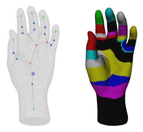
Figure 8.2 – Segmentation abstract graph and resulting segmentation.
