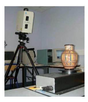
Figure 2.6 – Lab's Minolta VI-300 laser range scanner.
