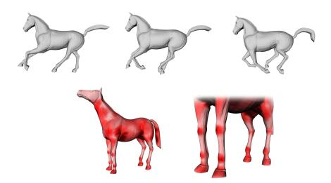
Figure 8.10 – Example frames of the horse dynamic triangulated surface (top row) and its quadratic edge-length deviation (bottom row).
