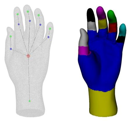
Figure 8.3 – Segmentation abstract graph (after perception heuristics based simplification) and resulting segmentation.
