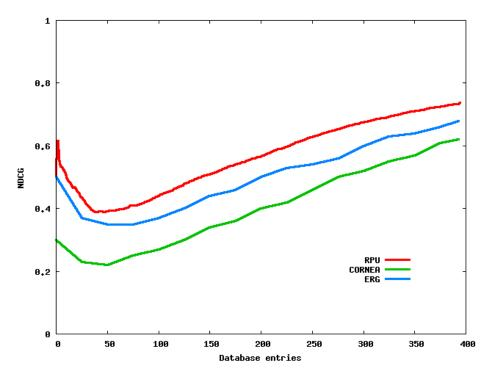
Figure 7.19 – Average Normalized Discounted Cumulative Gain (NDCG) vectors for Reeb pattern unfolding (RPU), (BMSF06) (ERG) and (CDS\*05) (CORNEA) on the SHREC 2007 data-set.
