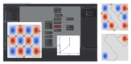
**Fig. 4** Results of the TTK-based Morse-Smale complex computation in Inviwo. The figure shows the underlying visualization pipeline (background), and Morse-Smale complexes for different simplification thresholds (foreground/right).
